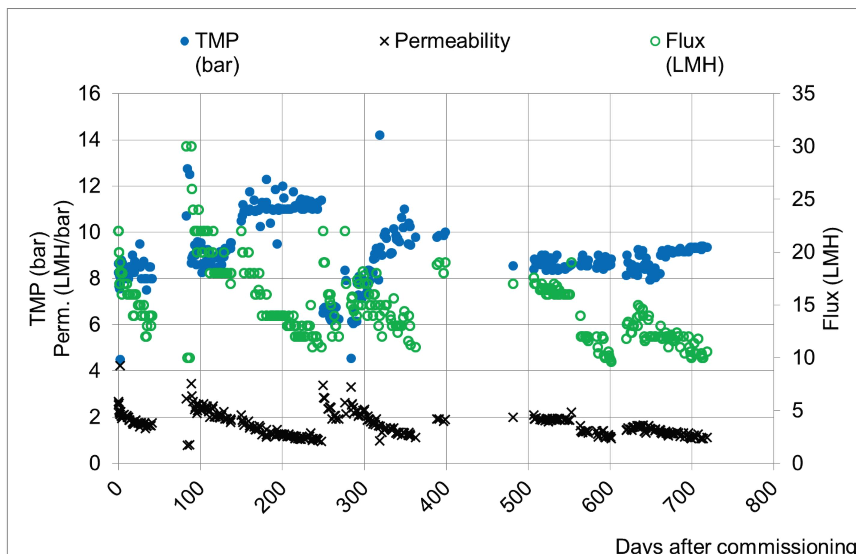
Figure 2. Registered parameters (TMP, permeability and flux) of the RO-unit
