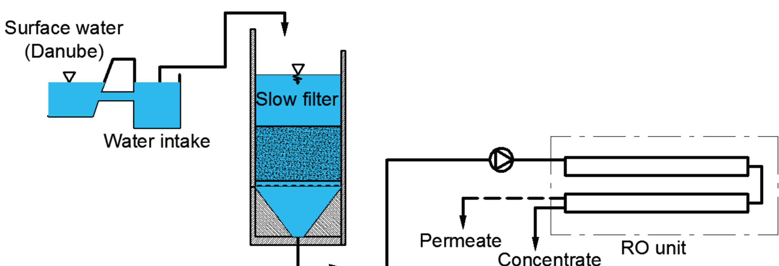
Figure 1. Scheme of RO unit fed with slow filtered surface water for RBF simulation
