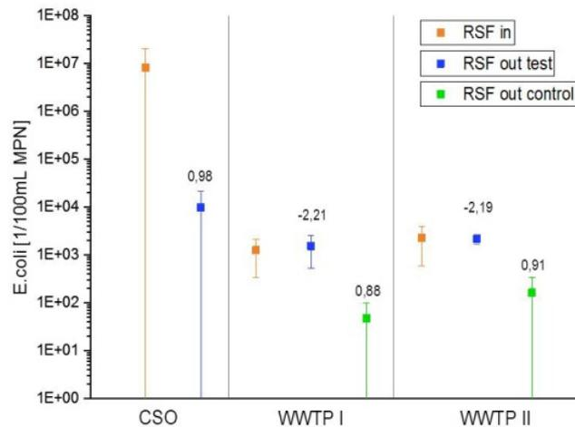
**Figure 37** Mean *E. coli* concentration in the in- and outflow of the CSO event, scenario I (WWTP I) and scenario II (WWTP II) on conventional pilot-RSF (without GAC; “out test”); “out control” equals to control-RSF (n=4).
