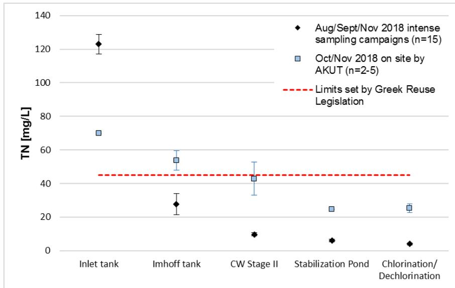
**Figure 13 TN concentration at different sampling points at WWTP Antiparos (average; standard deviation).** Intense sampling campaigns Aug/Sep/Nov: n=15 (black); Oct/Nov on site by AKUT: n=2-5 (blue), "Inlet tank" = effluent equalization tank and "CW Stage II" = CW Stage I for samples taken by AKUT; red line: limit for restricted irrigation.
