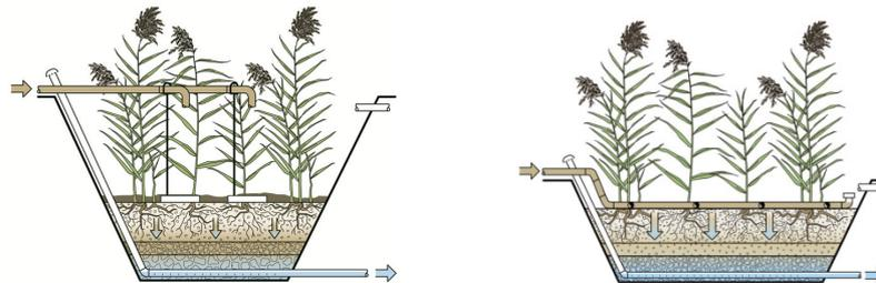
**Figure 3** Two-stage French system (left: first stage, right: second stage) (Dotro et al., 2017).
