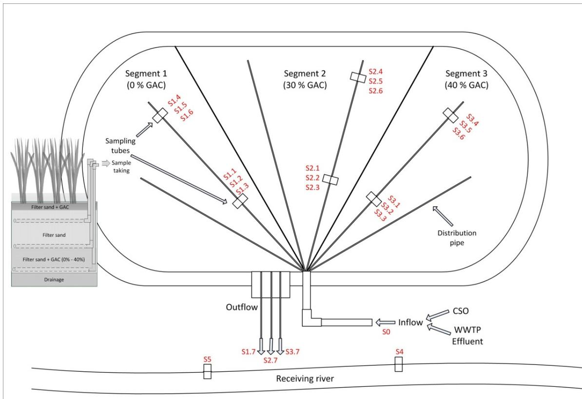
**Figure 31** Schematic view of the setup of the full scale demonstration site in Rheinbach.
