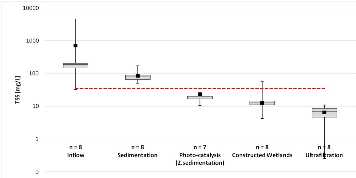
**Figure 22** Boxplots of TSS concentrations at different sampling points at WWTP Thirasia, Oct-Nov 2018. Boxplots with median, 25- and 75-percentil; black dots: average; whiskers: minimum and maximum; red line: limit for restricted irrigation.
