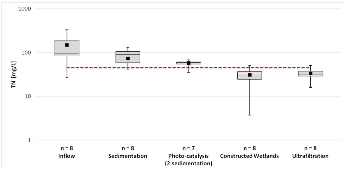
**Figure 23** Boxplots of TN concentrations at different sampling points at WWTP Thirasia, Oct-Nov 2018. Boxplots with median, 25- and 75-percentil; black dots: average; whiskers: minimum and maximum; red line: limit for restricted and unrestricted irrigation.
