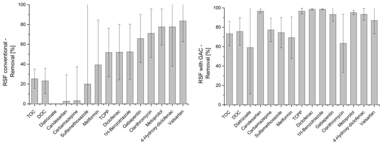
**Figure 33** OMP removal (%) in conventional RSF (left) and RSF with GAC (right). Columns: median; error bars: standard deviation; left: n=27-85, 09/2014 – 11/2018; right: n=14-56, 04/2015 – 11/2018; values < LOQ = LOQ.
