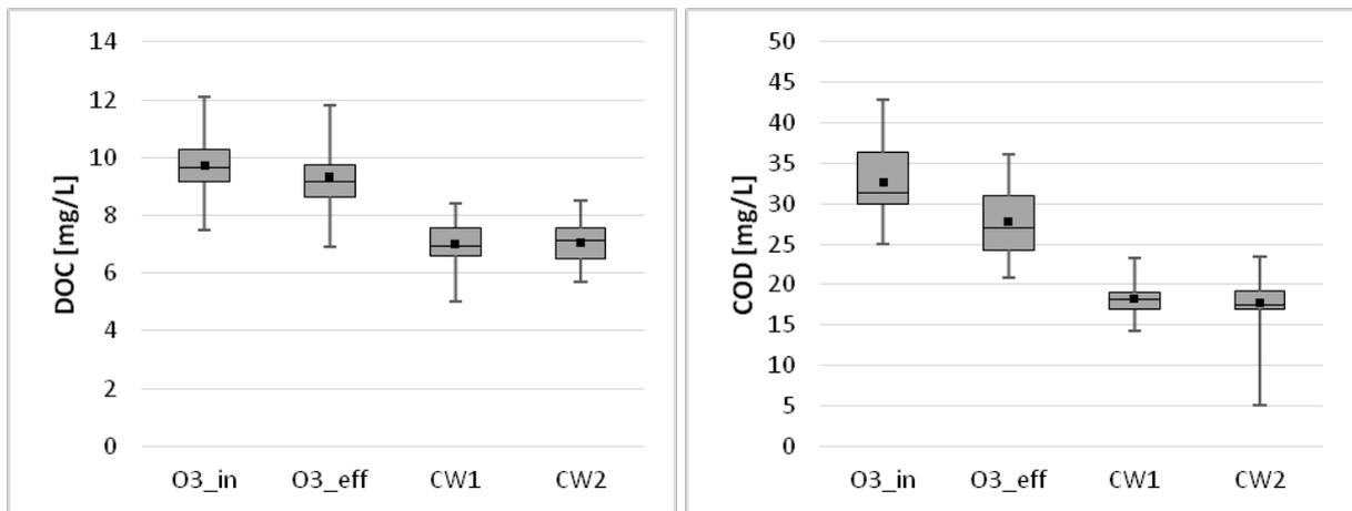
**Figure 40** Boxplots of DOC (left, n=22-34) and COD (right, n=22-24) concentrations at different sampling points. Boxplots with median, 25- and 75-percentile; black dots: average; whiskers: minimum and maximum.
