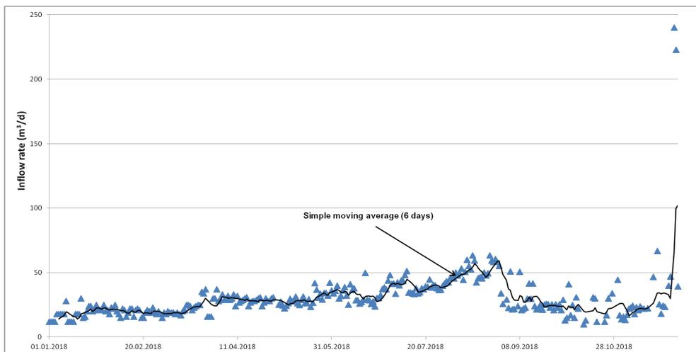
Figure 20 Inflow rate [ $\text{m}^3/\text{d}$ ] of the WWTP at Thirasia and a simple moving average (6 days) in 2018.
