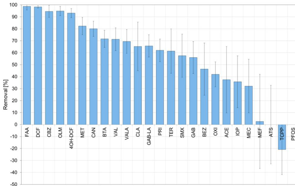
**Figure 45** Mean removals with standard deviations (n=8-41) of monitored OMP during ozonation calculated with conservative approach regarding LOQ. When effluent concentration was <LOQ the value of LOQ was used for calculation.
