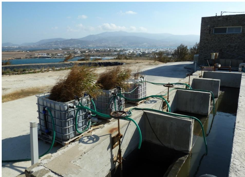
Figure 17 Test filter containers at outlet of Imhoff tank at WWTP Antiparos (Nov 2018).
