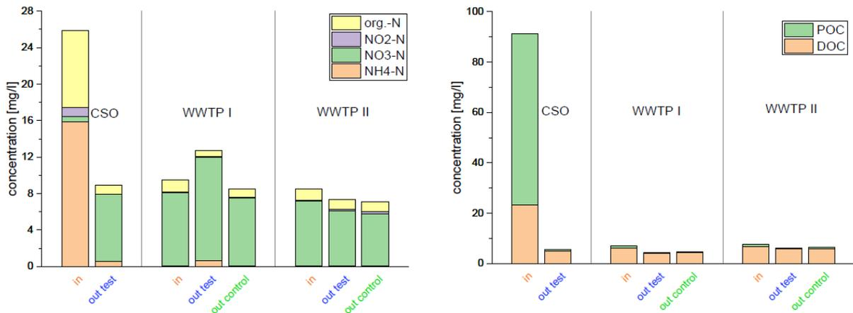
**Figure 36 Mean nitrogen (left), DOC and POC (right) concentration in the in- and outflow of the CSO event, scenario I (WWTP I) and scenario II (WWTP II) on conventional pilot-RSF (without GAC; “out test”); “out control” equals to control-RSF (n=4).**
