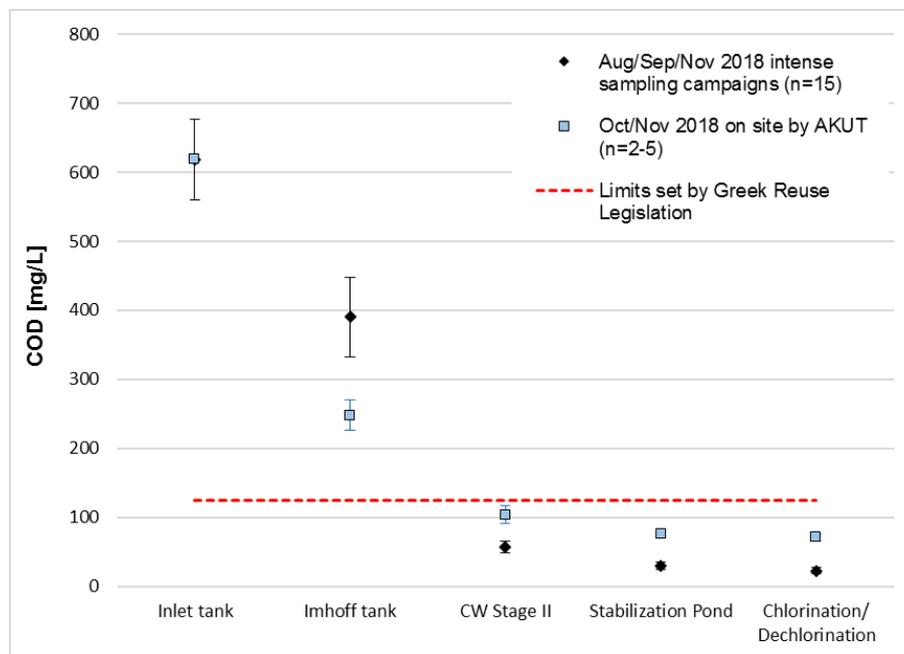
**Figure 10** COD concentration at different sampling points, WWTP Antiparos (average; standard deviation). Intense sampling campaigns Aug/Sep/Nov: n=15 (black); Oct/Nov on site by AKUT: n=2-5 (blue), "Inlet tank" = effluent equalization tank and "CW Stage II" = CW Stage I for samples taken by AKUT; red line: limit for restricted irrigation.
