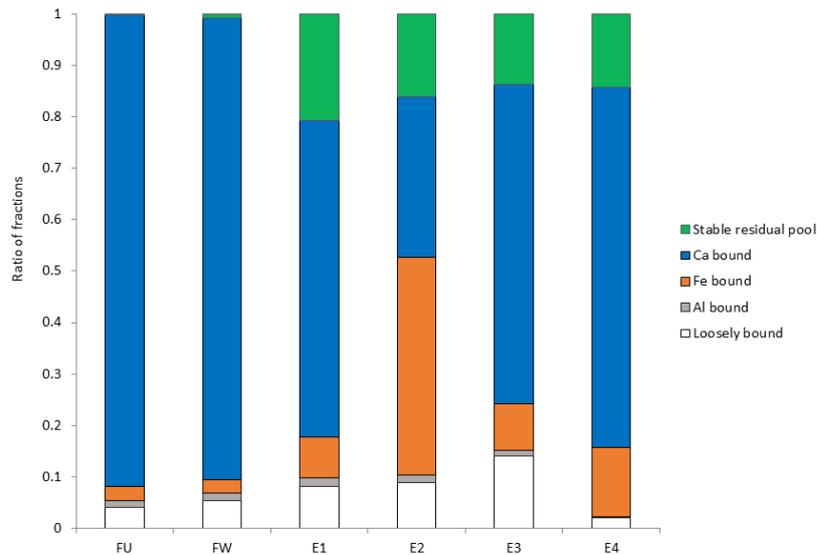
**Figure 62** Phosphorus sequential extraction from fresh media unwashed (FU) and washed (FW – rinsed with clean water to remove any loose deposits), and used media from four locations in the direction of the flow in the middle of the bed, with E1 closer to the inlet and E4 closer to the outlet.
