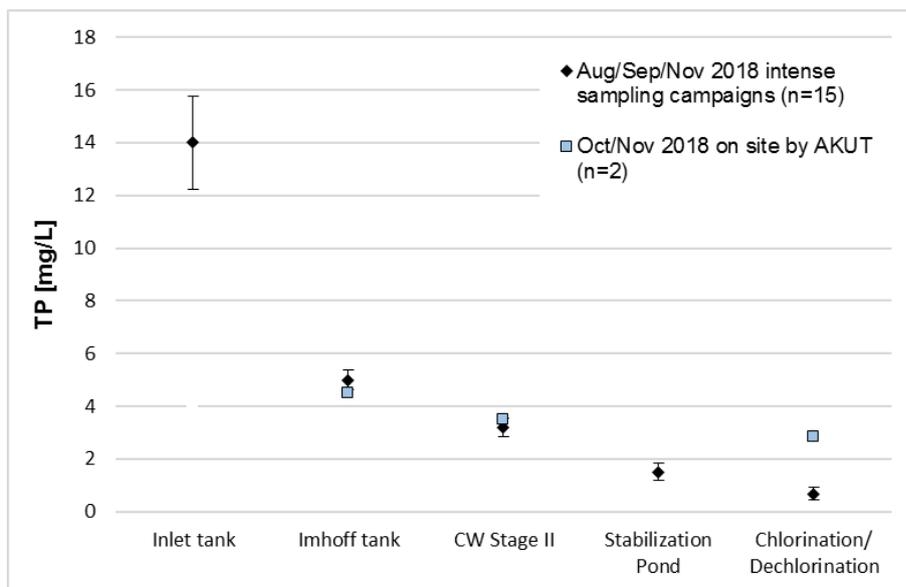
**Figure 14 TP concentration at different sampling points at WWTP Antiparos (average; standard deviation).** Intense sampling campaigns Aug/Sep/Nov: n=15 (black); Oct/Nov on site by AKUT: n=2-5 (blue), "Inlet tank" = effluent equalization tank and "CW Stage II" = CW Stage I for samples taken by AKUT.
