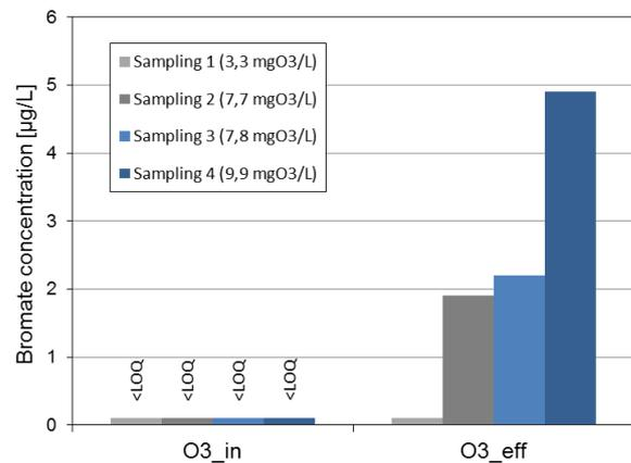
**Figure 48 Bromate formation at different O<sub>3</sub> doses.**
