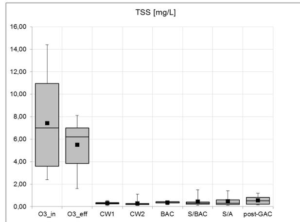
**Figure 44** Boxplots of TSS concentrations (n=8-20) at different sampling points. Boxplots with median, 25- and 75-percentil; black dots: average; whiskers: minimum and maximum.
