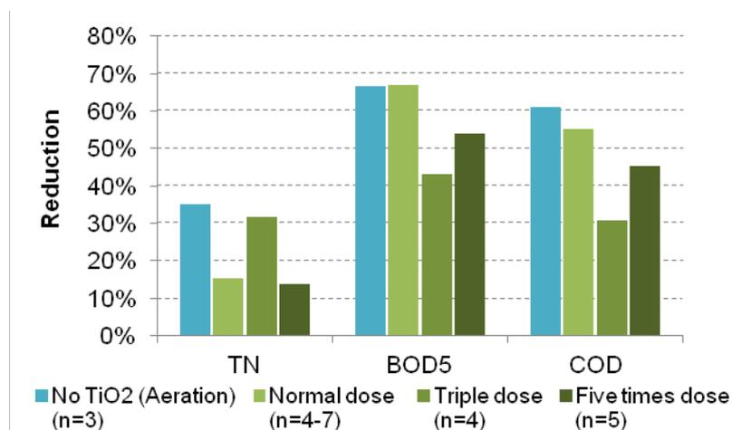
**Figure 28** Mean removal of TN,  $BOD_5$  and COD in the photocatalysis stage under different dosages of  $TiO_2$ . No  $TiO_2$ : Jul-Aug 2018; Normal dose (0.1  $kg/m^3$   $TiO_2$ ): Mar-Jun 2018; Triple dose (0.3  $kg/m^3$   $TiO_2$ ): Sep 2018; Five times dose (0.5  $kg/m^3$   $TiO_2$ ): Oct-Nov 2018.
