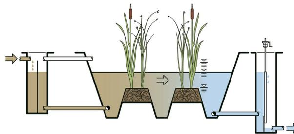
Figure 1 Overview schematic of FWS wetland (Dotro et al., 2017).
