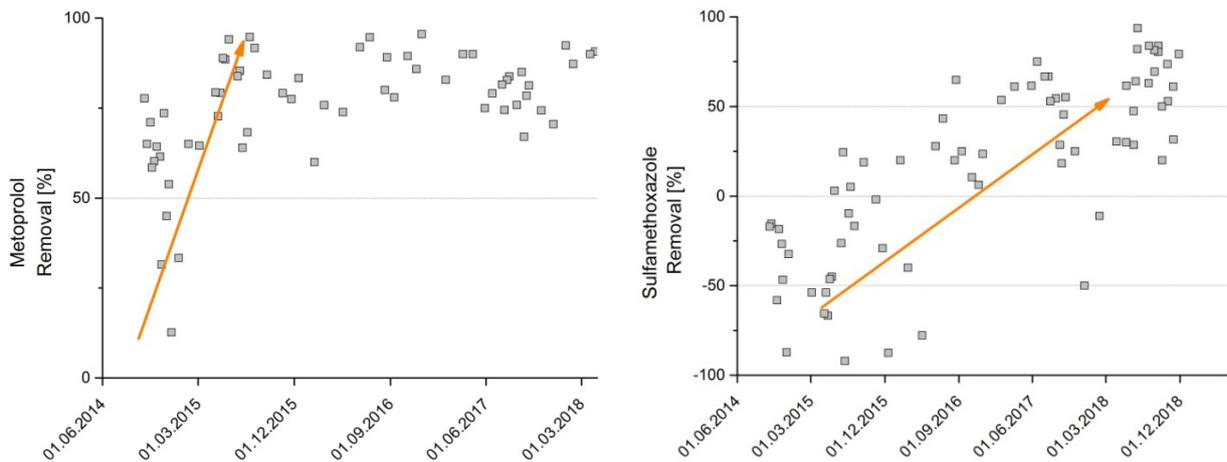
**Figure 34** Removal (%) of Metoprolol (07/2014–03/2018) and Sulfamethoxazole (07/2014–12/2018) in the conventional RSF.
