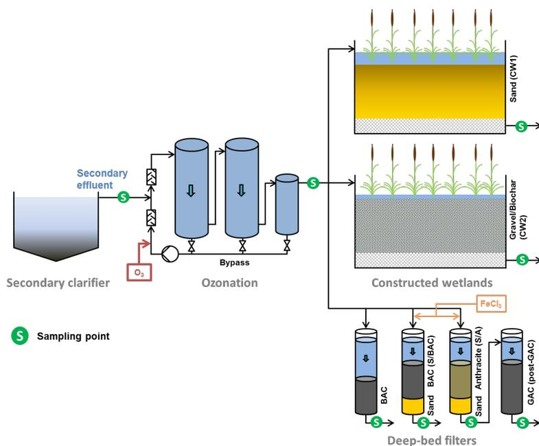
Figure 39 Pilot-plant flow scheme at WWTP Schönerlinde.
