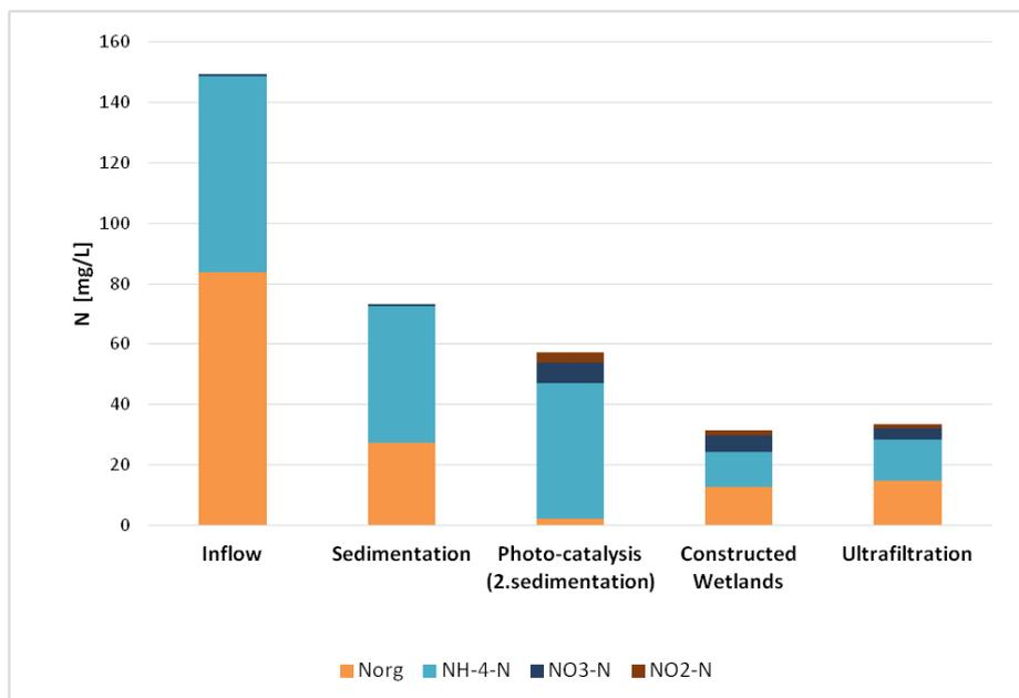
**Figure 24** Nitrogen fractions at different sampling points. Average values, n = 8, Thirasia, Oct-Nov 2018.
