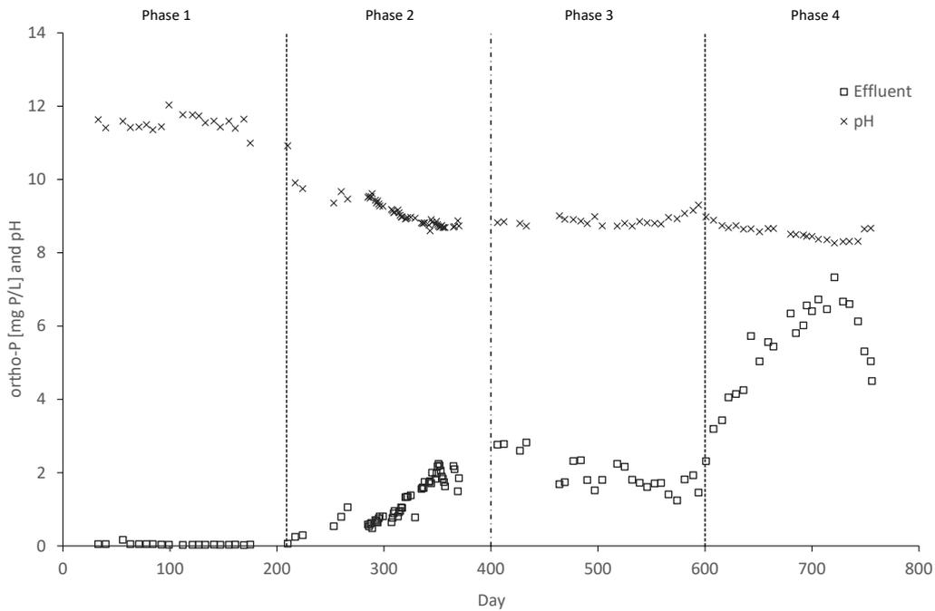
**Figure 56** Evolution of the effluent phosphorus concentration and pH over time.
