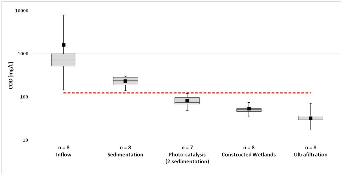
**Figure 21** Boxplots of COD concentrations at different sampling points at WWTP Thirasia, Oct-Nov 2018. Boxplots with median, 25- and 75-percentil; black dots: average; whiskers: minimum and maximum; red line: limit for restricted and unrestricted irrigation.
