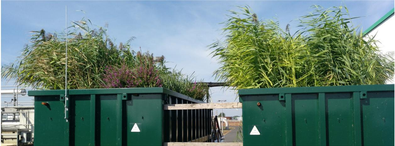
Figure 54 CW 2 (left container) with reed (left part) and sedge (right part), CW 1 (right container), Sept. 2018.
