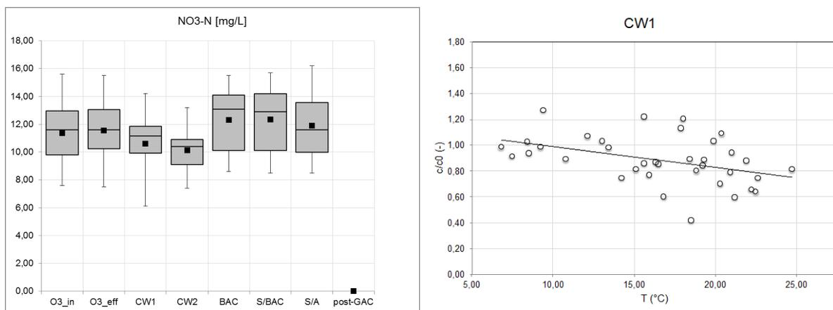
**Figure 43** Boxplots of  $\text{NO}_3\text{-N}$  concentrations ( $n=7-24$ ) at different sampling points (left); correlation of water temperature and  $\text{NO}_3\text{-N}$  reduction in CW1 (representative for both CW) (right). Boxplots with median, 25- and 75-percentil; black dots: average; whiskers: minimum and maximum. No data for post-GAC.
