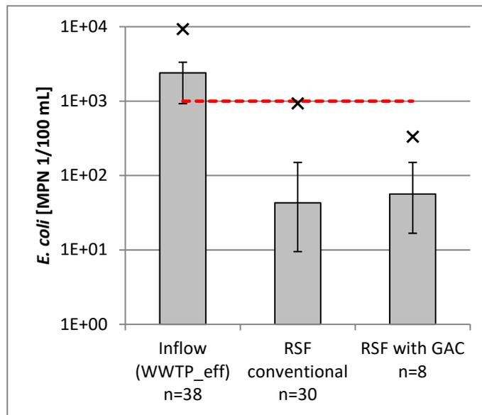
**Figure 35 Concentrations of *E. coli* at different sampling points; columns: median, error bars: 25<sup>th</sup> / 75<sup>th</sup> percentiles, crosses: 95<sup>th</sup> percentile.**
